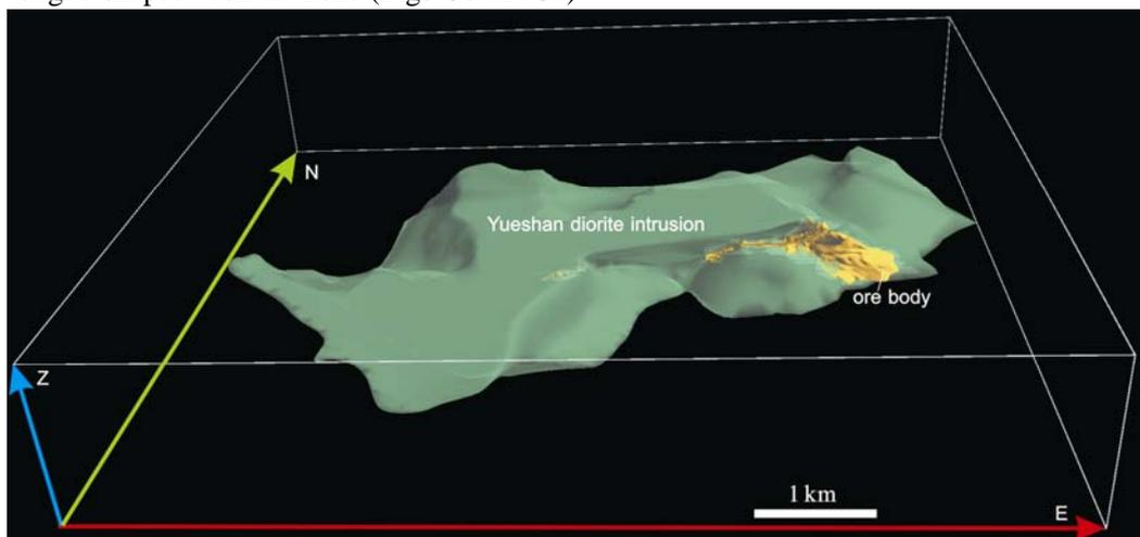
**Fig.2** 3-D shape modeling of the Yueshan intrusion and orebodies, by using of data from drillholes and geophysical surveying
