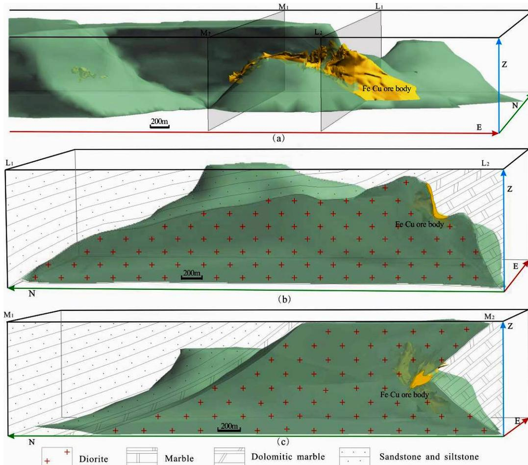
**Fig.3** 3D relationship of orebodies with shape of intrusion contact surface. (a) Entire view of eastern branch of intrusion and orebodies. (b) Cross section along L1-L2 and view toward east, showing typical “step-shaped” contact zone and orebody; (c) Cross section along M1-M2 and view toward east, showing typical “tongue-shaped” contact zone and orebody.
