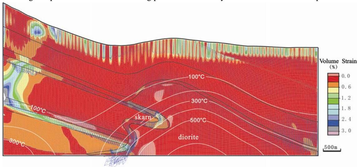
**Fig.4** Deformation, temperature and fluid flow results of Model A, showing Darcy fluid flow velocities (arrows), isotherms and total volume strain contour at 9,200 years, the maximum fluid flow velocity is  $3.262 \times 10^{-6}$  m/s.
