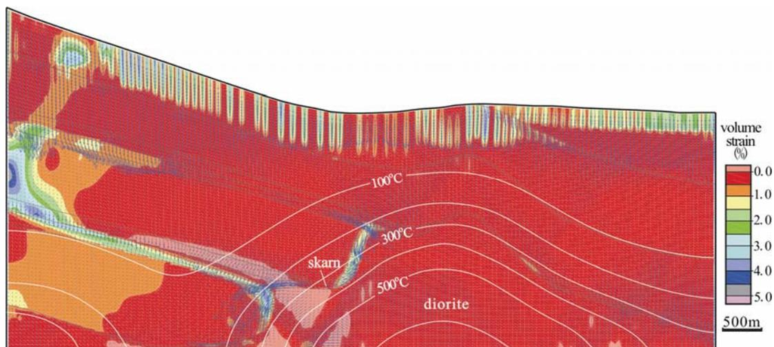
**Fig. 5** Deformation, temperature and fluid flow results of Model B, showing Darcy fluid flow velocities (arrows), isotherms and total volume strain contour at 6,000 years, the maximum fluid flow velocity is  $2.042 \times 10^{-6}$  m/s.
